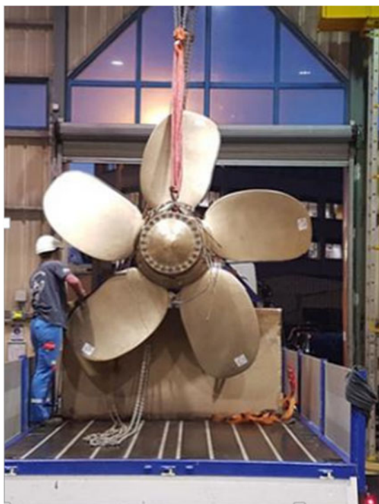
Fig. 2. 3D-printed screw of the new generation
