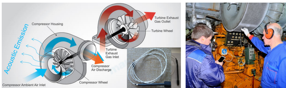
Figure 4. Recording the vibration of turbocharger using the EM-4015-BC electret microphone
